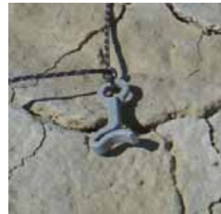
(Broken servo horn, Last year)
