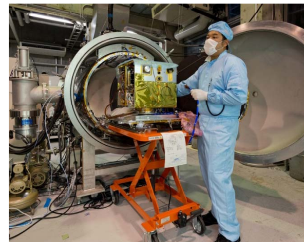
Thermal Vacuum Test of Uniform-1 FM
