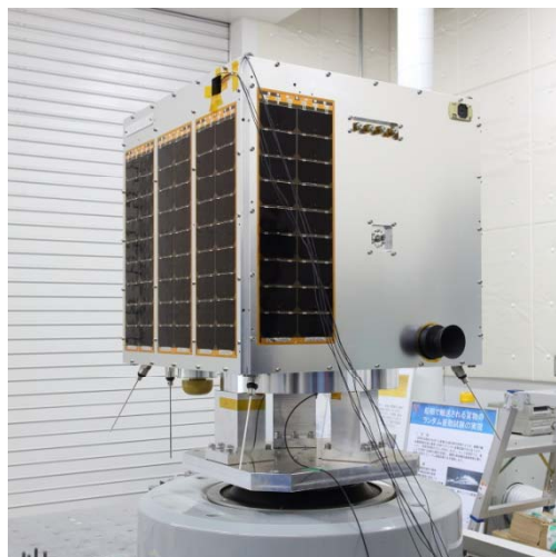
Hodoyoshi-1 FM and its Vibration Test and Thermal Vacuum Test
