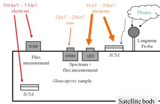
Fig. 7. Schematic of the Instruments for the Charging Mission.
