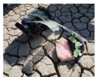
Because the separation mechanism had been damaged by the impact of the parachute deployment.
