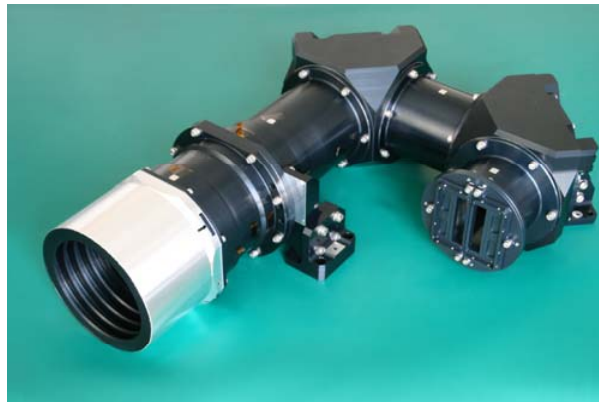
6.7m GSDO Refraction Optics
