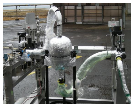
Fig. 14 Liquid hydrogen filling test.
