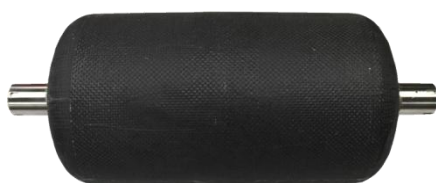
Fig. 13 Prototype liquid hydrogen tank.
