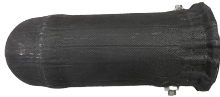
Fig. 15 Prototype liquid oxygen tank.
