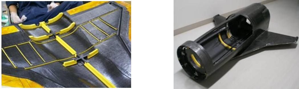
Fig. 9 Winged rocket structure made of CFRP.
