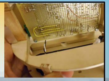
• Our Cansat is made of wood and each parts is combined by tight fit, like japanese traditional construction method, *"KUMIKI*".
